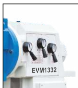
Vertical Speed Gear Box
