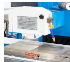
Grinding Head With Close Loop Magnetic Chuck
