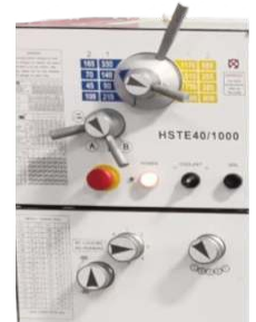
Speed & Feed Control Box with Metric, Imperial, Dp & module Thread Range
