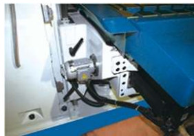
XYZ Central Lubrication for XYZ axis
