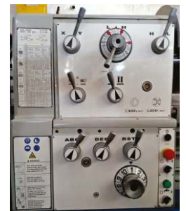
Speed & Feed Control Box with Metric, Imperial, Dp & module Thread Range
