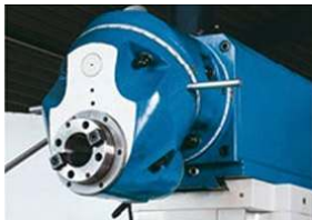
It Can Mill Any Angle Surface Through Front Half-sphere By Swivelling Milling Head
